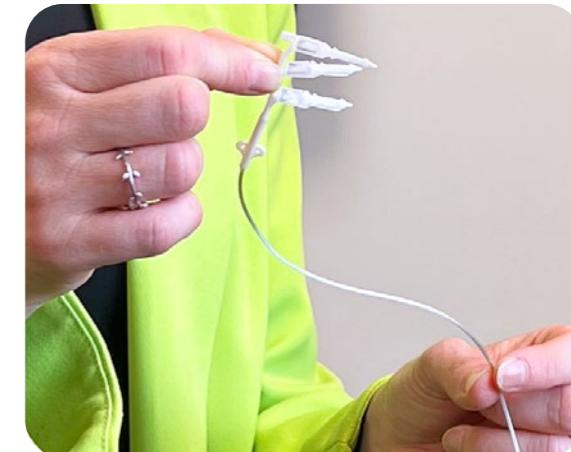
To overcome this limitation, Bionics Institute researchers have developed a device that stimulates the vagus nerve at the abdominal level, below the diaphragm, without side effects on the heart and lungs. This technology is called the abdominal Vagus Nerve Stimulation (aVNS) System, and the device is made up of an electrode array implanted on the vagus nerve via keyhole surgery that stimulates and records nerve activity.
